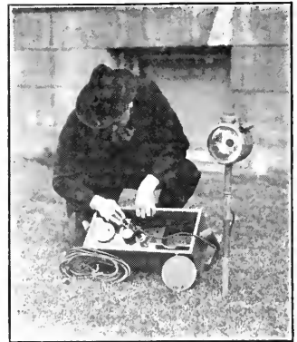
Fig. 7 —Trench Signalling Unit in operation
